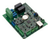
Door Controller LAN/ RS485
