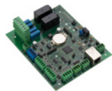
Door Controller LAN/ RS485
